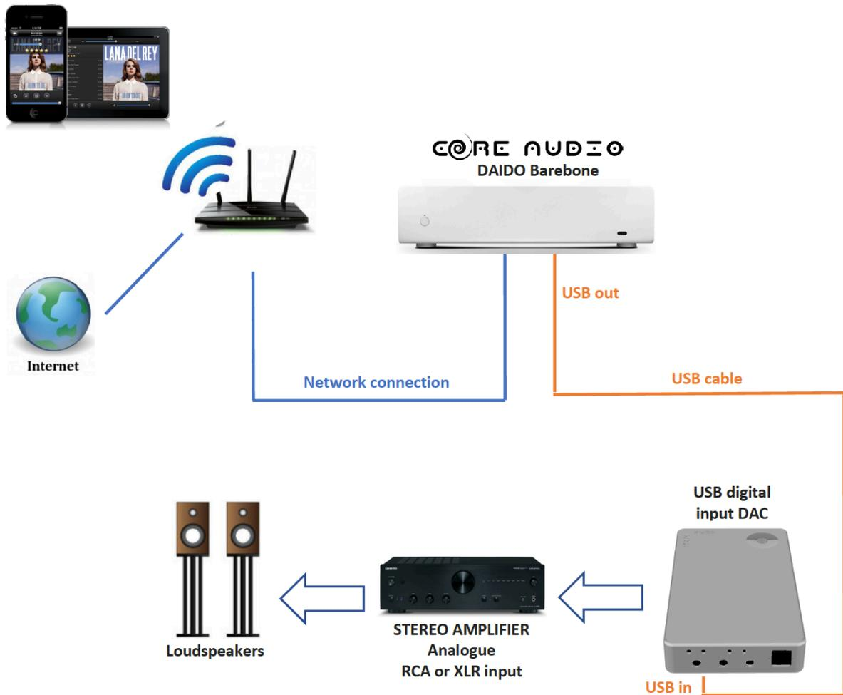
In this case the User aren't use a separated USB/SPDIF converter. The Music server is connected directly with USB cable to the DAC.
