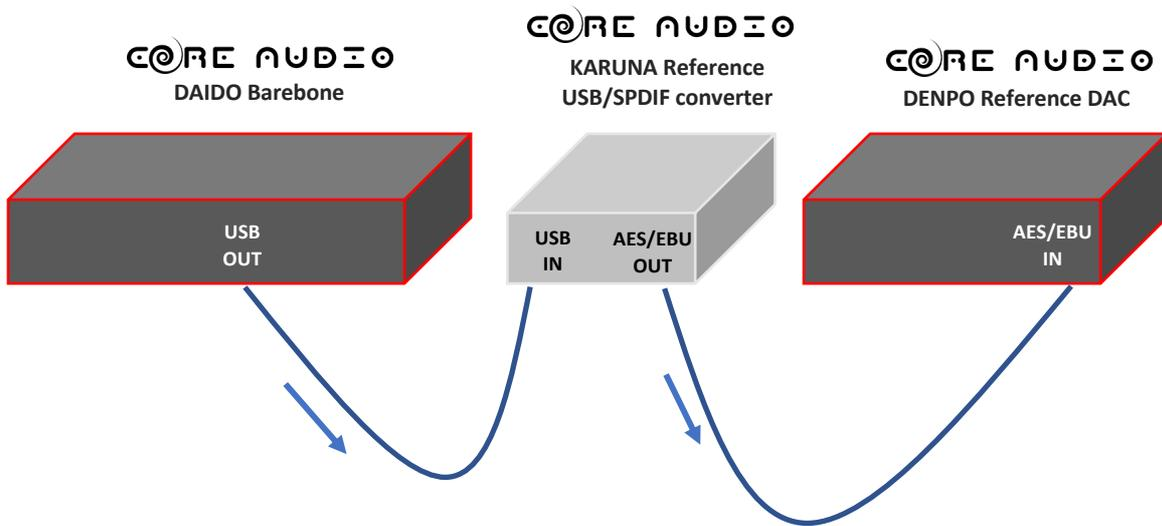
Digital coax connection: with S/PDIF connecting cables
