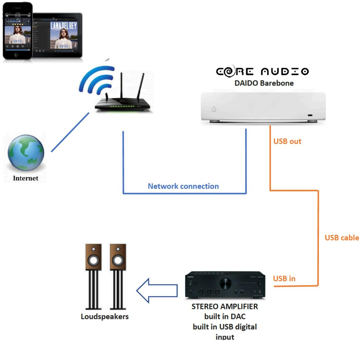
A frequent case when the User want to use a fully integrated devices, for example Stereo Integrated Amplifier's built in DAC with digital USB input. In this case the User can connect his music server directly via USB to the Stereo Amplifier.
